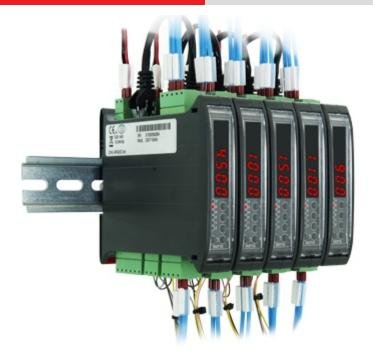
Compact, multifunction weight transmitter / indicator, for panel mounting on DIN bar. It allows the direct reading and diagnostics of the connected weighing system. The wide range of available interfaces, makes it easy to integrate the weighing with any automation system. CE-M approved (OIML R-76 / EN 45501). MID approved (OIML R-61).
