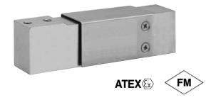
bench and counting scales. For wash-down protection an optional IP65 encapsulation protection is available. Constructed from stainless steel this high accuracy load cell is approved to Factory Mutual and other stringent approval standards.
