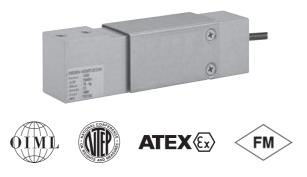
Available in anodized aluminum these high accuracy load cells are approved to NTEP and other stringent approval standards, including OIML R60. For hazardous environments this load cell has EEx ia IIC T4 level of approved option. An optional special humidity resistant protective coating assures long-term stability over the entire compensated temperature range.
