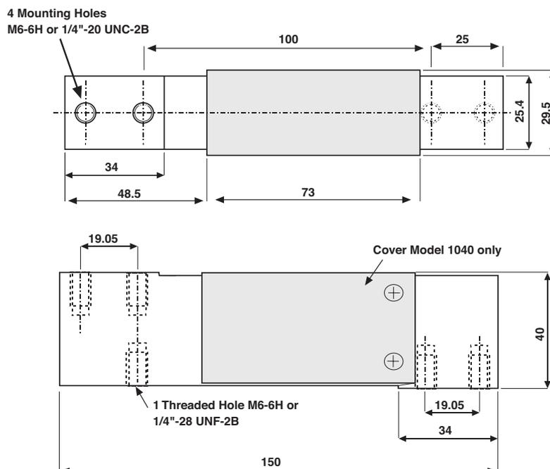
Low Capacity Single-Point Aluminum Load Cells
