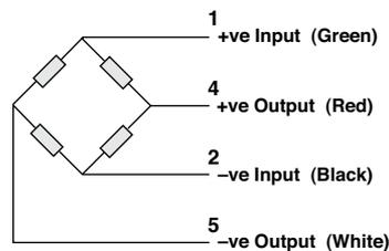
The load cell is provided with a 4 conductor ribbon cable and with optional AMP#103957-4 connector
